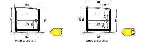
CCS – cover | single, curved | sliding (sideways) CCP – cover | single, curved | sliding (slide-up/push)
